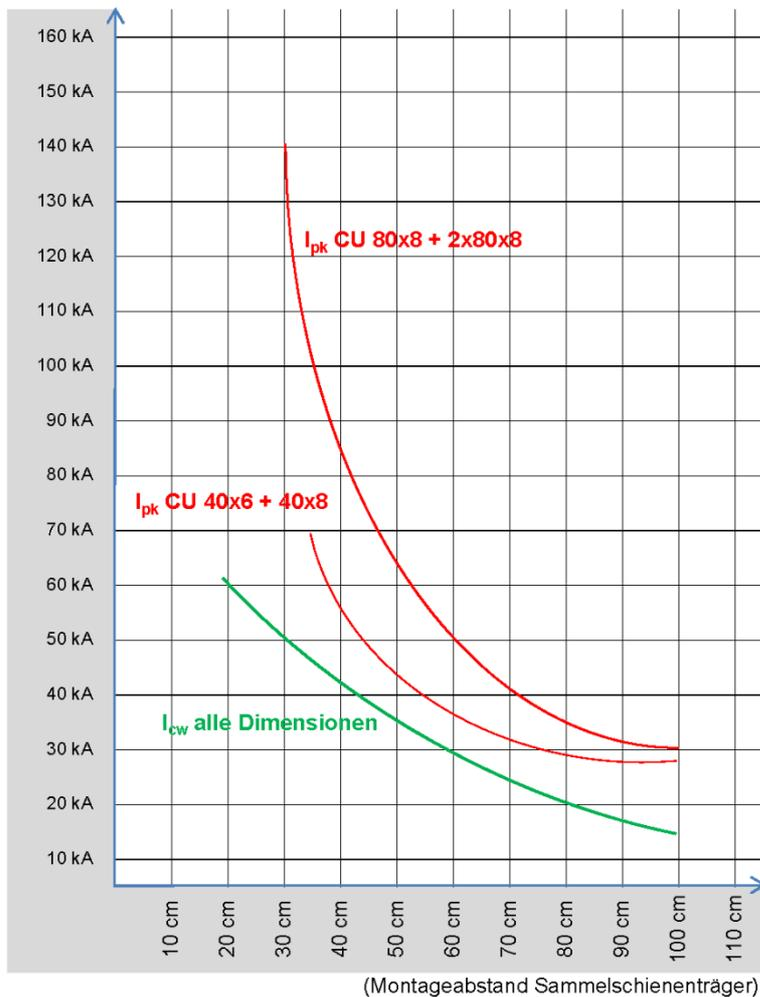
$I_{pk}$ : Bemessungsstromfestigkeit (rated peak withstand current) / 0.1s
